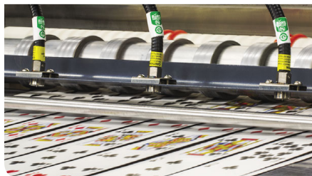
Gen4 Ionizing Points remove static from a card slitting operation.
