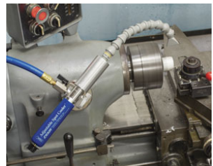
The Adjustable Spot Cooler maintains critical tolerances on machined plastic parts.
